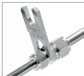
Properly tightened, the gauge will not fit
